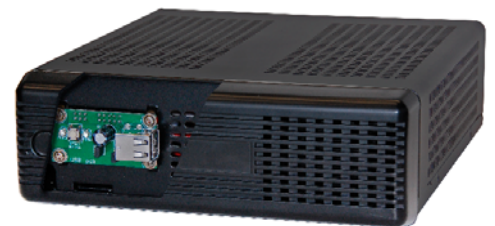
USB 2.0 Ports concealed under front cover are ideal for the installation of hardware license keys or wireless network (Bluetooth / WiFi) adapter cards
